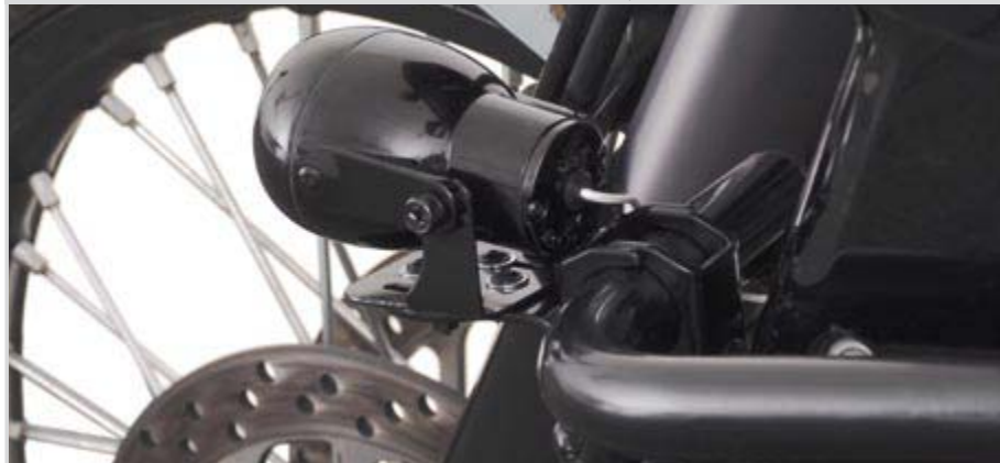
Fog Light Kit mounted on crashbar with Fog Light Clamp Set.
