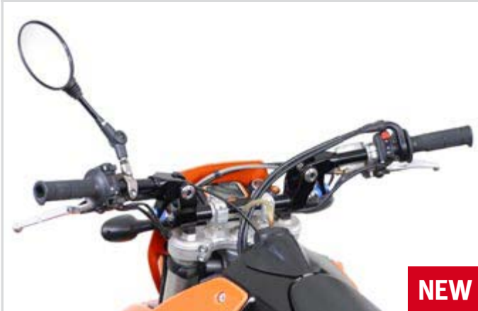
Nonshock Endurance Bar mounted on streetfighter motorbike.
