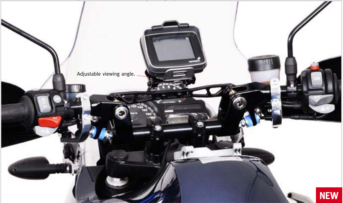
Vibration and shock absorption of Nonshock Endurance Bar.
