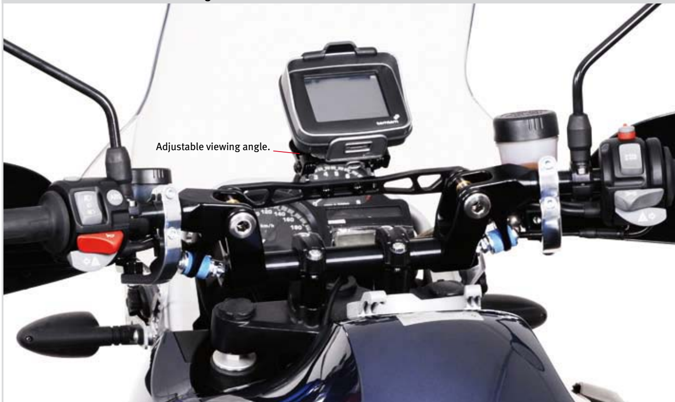
Vibration and shock absorption mounting of GPS on Nonshock Endurance GPS-Mount.
