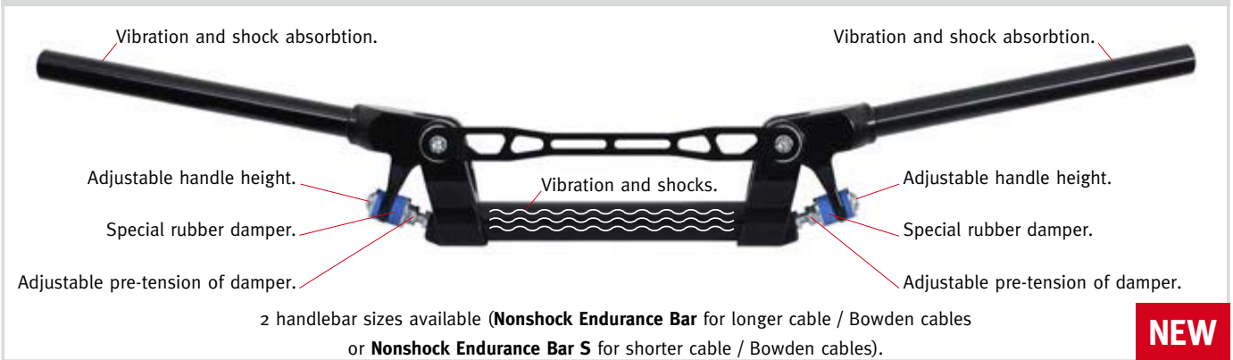
Vibration and shock absorption of Nonshock Endurance Bar.
