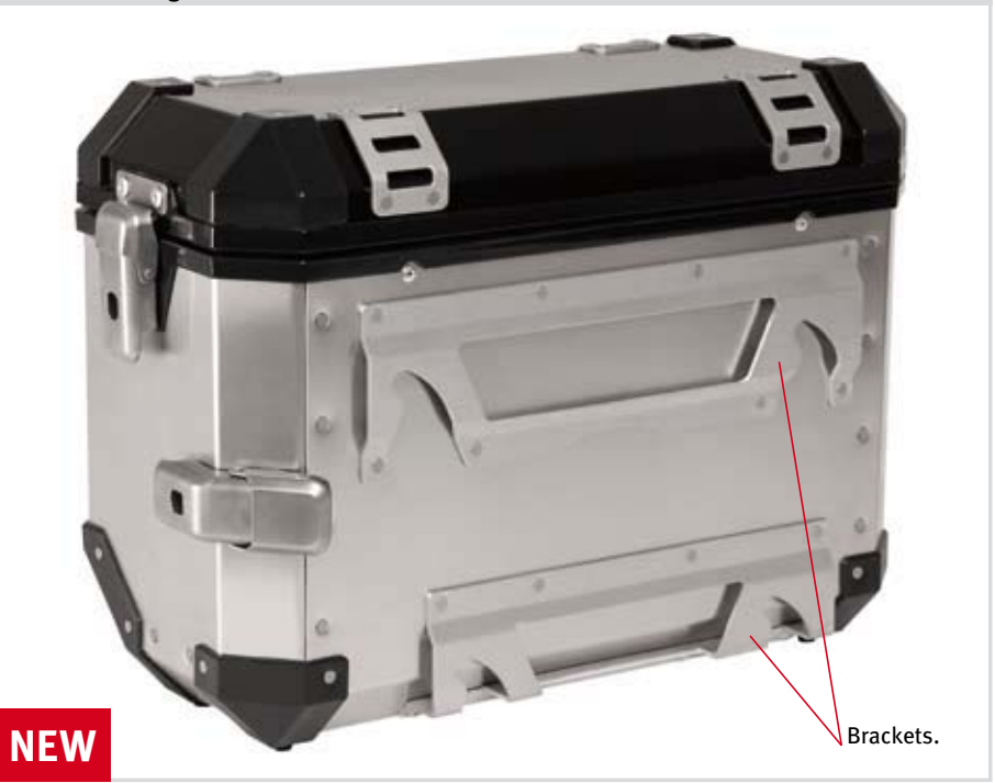
These mounting brackets attach TraX® EVO to QUICK-LOCK Side Carriers.
