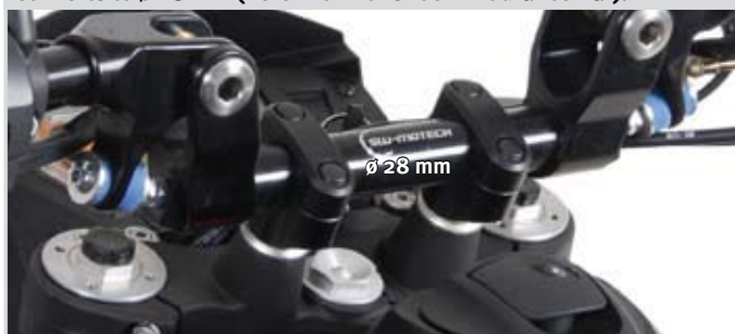
Converts to ø 28 mm (here with Nonshock Endurance Bar).
