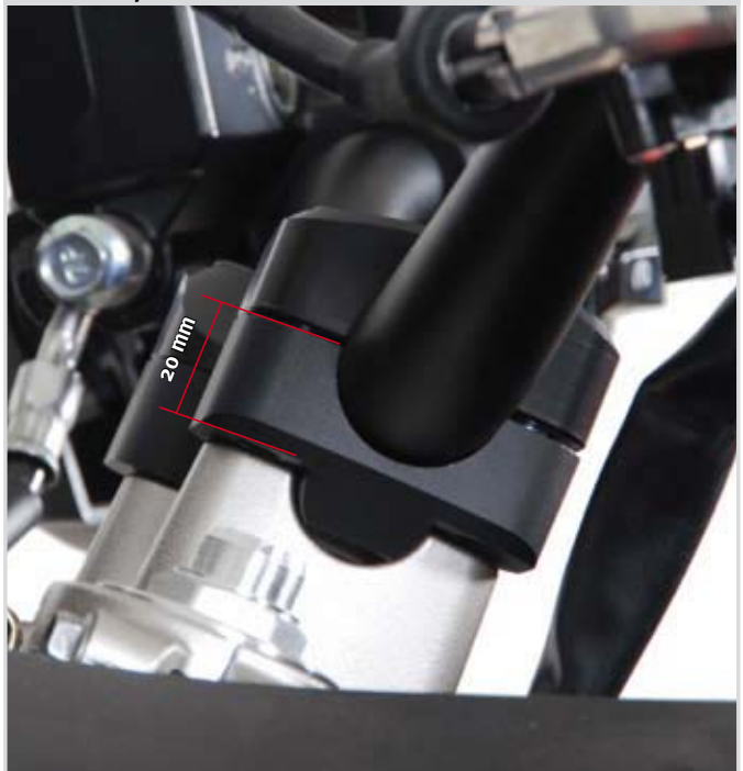
Raises bar position 20 mm.
